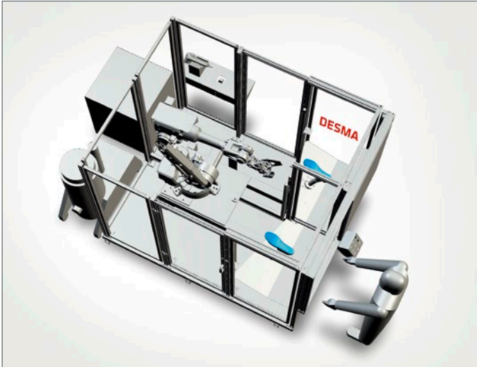
2 STATION ROUGHING CELL
